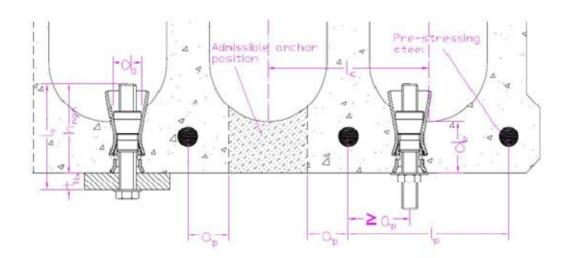
h<sub>nom</sub>: Overall anchor embedment depth in the base material
